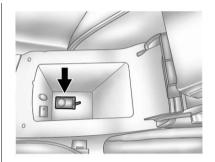
4. Place the new transmitter into the transmitter pocket. The transmitter pocket is inside the center console storage area located between the driver and front passenger seats. The storage area will need to be opened and the storage tray lifted up to access the transmitter pocket.
